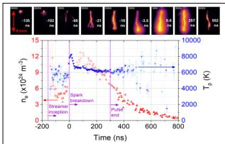
$\label{eq:Fig. 1. Evolution discharge morphology (top) and of $n_e$ and $T_p$ (bottom) from ignition until extinction.}$
